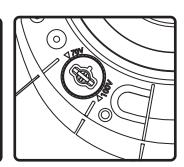
**7.** Adjust tap switch to proper setting. Switch is preset to maximum tap setting in 70.7 V mode (33 W)
