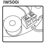
**4.** Connect speaker wires to terminals on rear of speaker.
