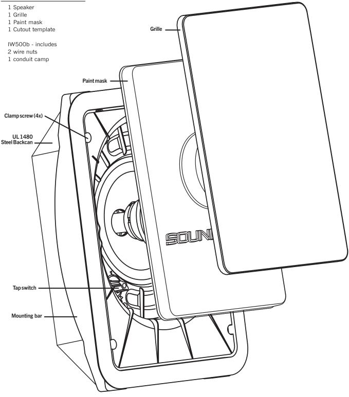
IW500b: Steel signaling speaker enclosure listed UL 1480
