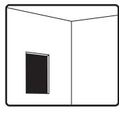
**2.** Use provided cut out template to make hole. Use Rotozip or other tool to cut hole in wall. Hole size, 7.5" x 10.75"
