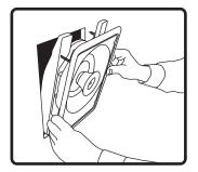
**5.** Insert speaker in to hole (bottom first) with mounting bar on inside of wall.
