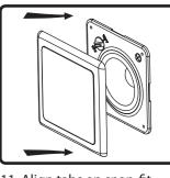
11. Align tabs on snap-fit grille with slots in baffle, gently press grille into place.
