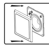
9. Align tabs on snap-fit grille 10. Done! with slots in baffle, gently press grille into place.
