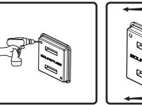
7. Insert speaker in hole. Tighten the two clamping screws. DO NOT OVERTIGHTEN
