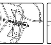
6. If required, attach seismic restraint system to the hole in the metal clamping arm, then to reinforced structure (safety cable not included).
