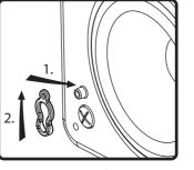
8. Attach grille safety clip by placing the large end of the clip over snap-fit post (1), then sliding clip until small end snaps into place around post (2).
