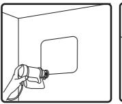
2. Use provided cutout template to mark hole. Use RotoZip or other tool to cut hole in wall. Hole size: 4.25 in. (108 mm) tall x 4.25 in. (108 mm) wide.
