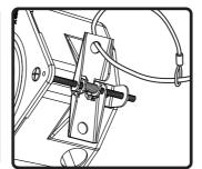
4. If required, attach seismic restraint system to the hole in the metal clamping arm, then to reinforced structure (safety cable not included).
