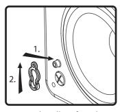
10. Attach grille safety clip by placing the large end of the clip over snap-fit post (1), then sliding clip until small end snaps into place around post (2).
