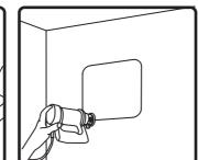
1. Unpack speaker. Leave paint mask in place until after speaker is installed or painting is complete.
