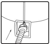
3. Feed speaker wires through conduit clamp and connect with wire nuts. Push wire nuts into backcan and affix conduit clamp.
