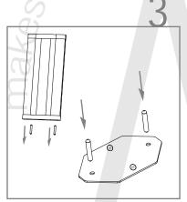
Remove the threaded sockets inside the panel and attach it on the base.
