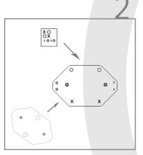
After, flip the base to attach the base stickers as shown on figure.
