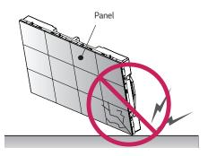
If the product is tilted onto the edge of the panel, the panel may be damaged.
