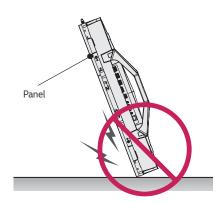
If the product is tilted onto the bezel, the bottom of the panel may be damaged.
