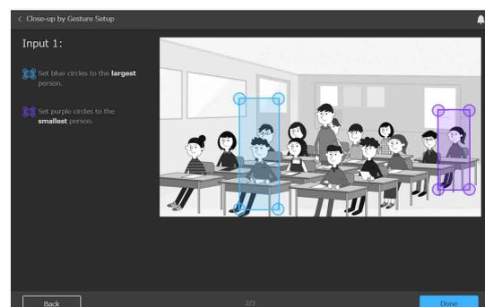
Set the maximum size and minimum size of the screen that would be fully occupied by a person when standing.
