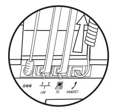
**2.** Align the protrusions on the bracket with their corresponding holes in the phone.
