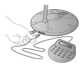
Figure 13. Connecting external dial pad
