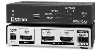
The Extron HDMI DA2 is a one input, two output HDMI distribution amplifier. It features EDID Minder<sup>®</sup> and Key Minder<sup>®</sup>, two Extron-exclusive technologies that automatically manage EDID communication and HDCP negotiation for reliable operation in commercial AV applications. The HDMI DA2 is ideal for applications that require the distribution of an HDMI source signal to two displays.
