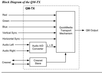
NOTE: The QM-TX is compatible with 2-Series control systems only.
