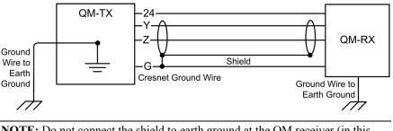
**NOTE:** Do not connect the shield to earth ground at the QM receiver (in this example, the QM-RX)
