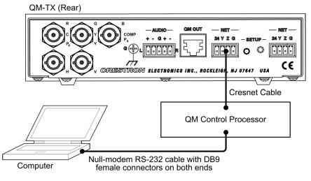
**NOTE:** Use a standard DB9 "Null-Modem" RS-232 cable when communicating with a QuickMedia control processor. Use a straight through cable when communicating with a 2-Series control processor.
