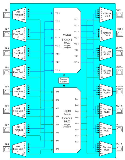
Up to two tiers of QM-MD8X8s can be cascaded to provide up to 64 QM inputs through one QM-MD8X8 as shown in the following block diagram.
