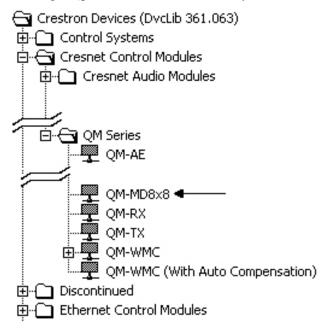
• The system tree of the control system displays the device in the appropriate slot with a default Net ID of 32 as shown in the following illustration.
