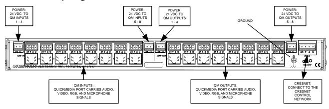
**NOTE:** Ensure the unit is properly grounded.
