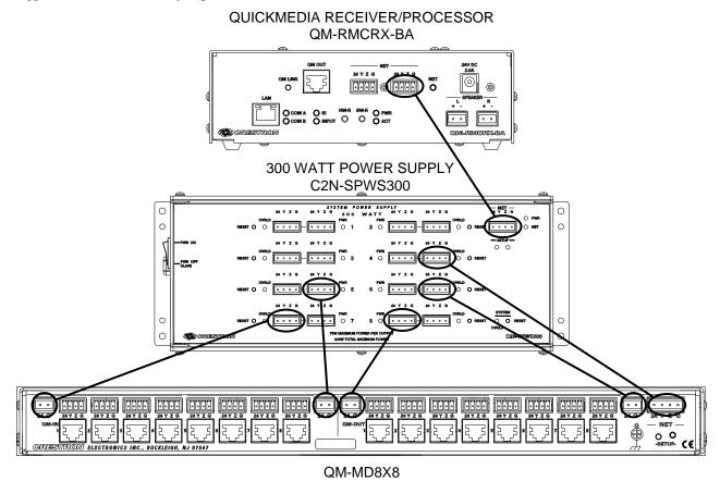
**NOTE:** The QM-MD8X8 can only be powered by the 4-position terminal block connector labeled **NET**.
