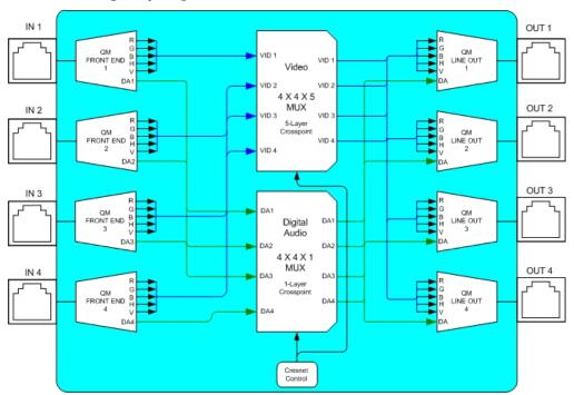
Up to two tiers of QM-MD4X4s can be cascaded to provide up to 16 QM inputs through one QM-MD4X4 as shown in the following block diagram.
