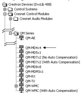
• The system tree of the control system displays the device in the appropriate slot with a default Net ID of 32 as shown in the following illustration.
