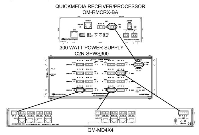
**NOTE:** The QM-MD4X4 can only be powered by the 4-position terminal block connector labeled "NET".
