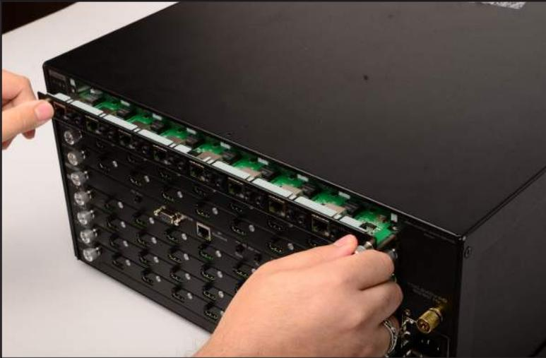
8. Secure the card by hand-tightening the fastening screws. Do not overtighten the screws. To prevent damage to the screws, do not use pliers or other high-torque devices.
