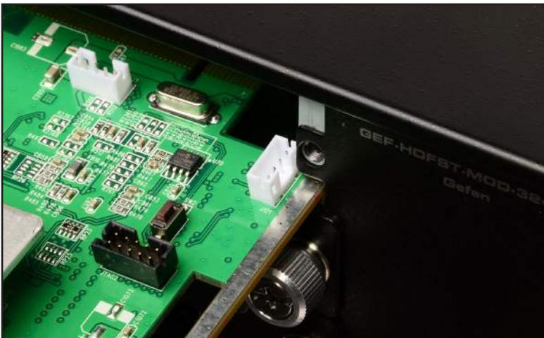
7. Position either hand on both sides of the matrix and firmly push the card with both thumbs until it snaps in place.
