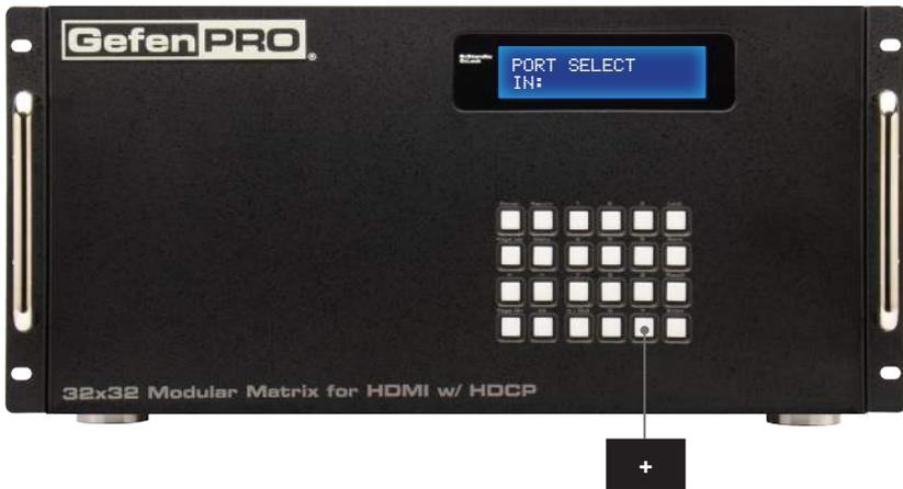
2. The front panel display will indicate that routing mode is active.
