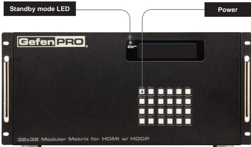
Standby mode is similar to powering-off the matrix. However, in standby mode, the matrix can be powered-on by executing the `#power` command. See [RS-232 and IP Configuration](#) for more information on using the RS-232 / IP commands.
