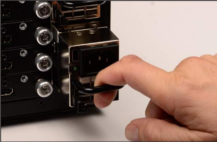
6. Gently push the new power supply into place. The power supply will snap into place once it is fully installed.
