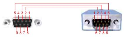
Only Pins 2 (RX), 3 (TX), and 5 (Ground) are used on the RS-232 serial interface
