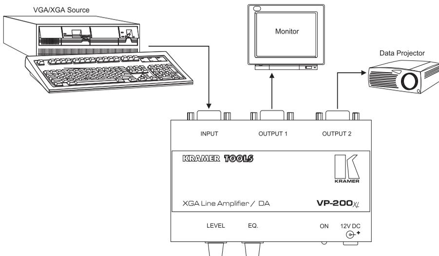
Figure 2: A typical application of the VP-200xl
