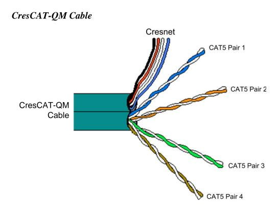
**NOTE:** Do not untwist the two wires in a single pair for more than 1/3-1/2" (8–12 mm) when making a connection. The twists are critical to canceling out interference between the wires.
