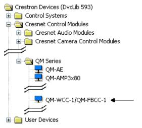
The system tree of the control system displays the device in the appropriate slot with a default Net ID as shown in the following illustration.
