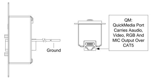
**NOTE:** Ensure the unit is properly grounded by connecting the ground wire to an earth ground (building steel).
