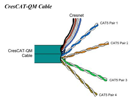
**NOTE:** Do not untwist the two wires in a single pair for more than 1/3-1/2" (8 - 13 mm) when making a connection. The twists are critical to canceling out interference between the wires.
