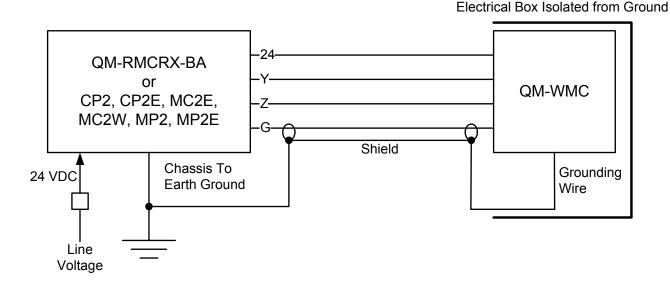
**NOTE:** When the Cresnet shield is used to connect the QM-WMC/WMC-VCC/WCC-2 to the ground terminal of a PRO2, PAC2, AV2 or any other 2-Series control system where the chassis is already earth grounded, the grounding wire from the control system to earth ground is unnecessary.
