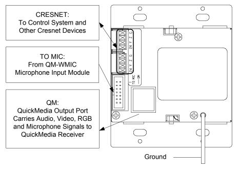
**NOTE:** Ensure the unit is properly grounded. Refer to step 4 on page 26.
