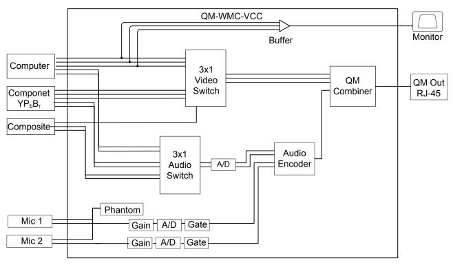
Internal Block Diagram of the QM-WMC-VCC (with QM-WMIC)
