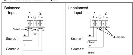
Typical Balanced/Unbalanced Inputs
