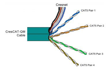
**NOTE:** Do not untwist the two wires in a single pair for more than 1/3-1/2" 8 - 13 mm) when making a connection. The twists are critical to canceling out interference between the wires.
