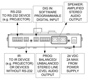
Hardware Connections for the QM-RX1-2G (Bottom View)
