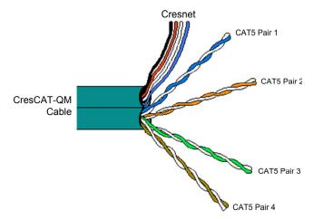
**NOTE:** Do not untwist the two wires in a single pair for more than 1/3-1/2" (8-12 mm) when making a connection. The twists are critical to canceling out interference between the wires.
