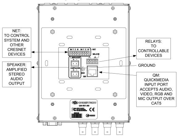
Hardware Connections for the QM-RX1-2G (Rear View)
