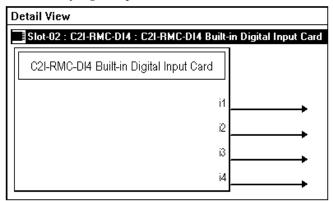
The C2I-RMC-DI4 provides four digital inputs for connection of external sensors or other contact closure devices. The <i>outputs are a logical high until it detects the presence of a low on the corresponding input.
