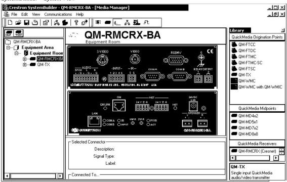
7. Setup QM network cable routing. Right-click on the connector and select the routing to the desired device.
