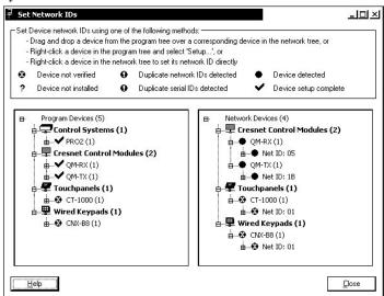
SystemBuilder detects all connected devices and displays a graphic that verifies all devices and indicates the status of the hardware and software Net IDs.
