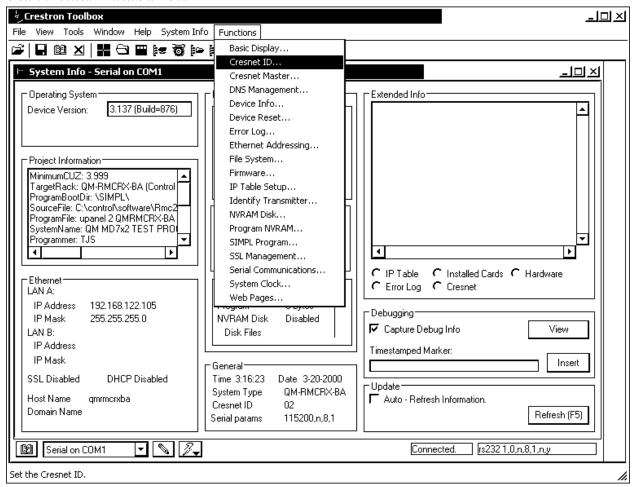
Select the new Net ID from the pull-down list. Ensure that the new hardware ID agrees with the ID assigned in SystemBuilder and is not a duplicate.
