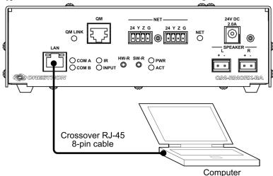
Once the cable connections are made, open Crestron Toolbox. Click
