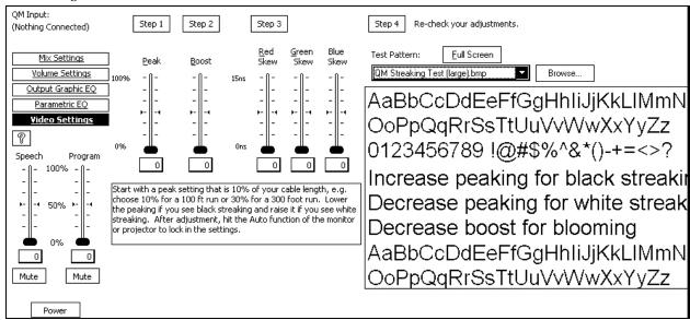
Step 1 – If the text is blurred and the text color persists (smears) into the blank space after the text, this is "black streaking" and you need to increase the peaking value. If you see white bands persisting after the text or you see small white areas after the text, you have "white streaking" and you need to decrease the peaking value.
