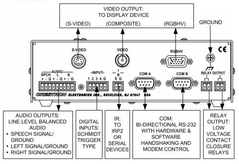
**NOTE:** COM B is shared for device control and serial console connection.
