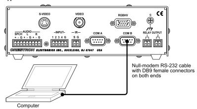
1. Open Crestron Toolbox and click **Tools** | **Manage Address Book** to display the communications settings. Enter the new address name, and then click **RS-232** as the connection type.
