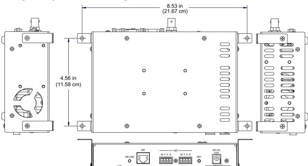
Mounting Positions of the Four Included Mounting Brackets
