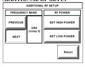
Press the **ADDITIONAL SETUP** button to display the ADDITIONAL RF SETUP screen. In situations where two or more touchpanels are in close proximity and could conflict with each other, press the **SET LOW POWER** button to reduce the touchpanel's power and minimize the possibility of interference. The factory default setting is **SET HIGH POWER**.
