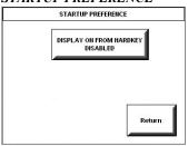
The Startup Preference feature allows (when the touchpanel is off or in standby) the display to come on or stay off when a "quick" pushbutton is pressed. From the SETUP MENU, press the **Startup Preferences** button to open the STARTUP PREFERENCE screen. In either case, the button signal will be sent to the RF gateway if the touchpanel is in standby mode.
