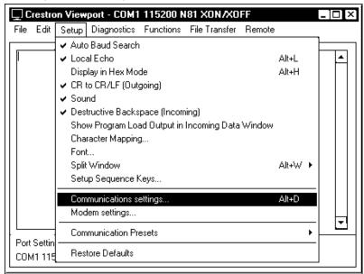
7. Select the **RS-232** connection type. Verify the available COM is selected. Verify that the baud rate is set to **115200** (PRO 2 default), the parity is **None**, the data bits is **Eight**, the stop bits is **One**, XON/XOFF is not selected, and RTS/CTS *is* selected. Click the **OK** button to save the settings and close the window.
