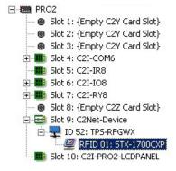
Double-click the TPS-RFGWX icon in the upper pane to open the "Device Settings" window. This window displays TPS-RFGWX device information. Select the *Net ID* tab to change the gateway Net ID, as shown in the following graphic.
