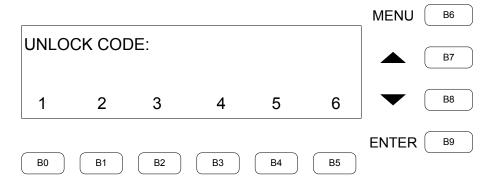
To unlock the front panel, enter the four-number numeric password with the **B0** through **B5** keys and then press **ENTER**.
