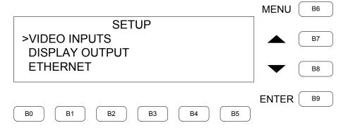
The SETUP menu provides access to five other menus: "VIDEO INPUTS", "DISPLAY OUTPUT", "ETHERNET", "CONTROL", "QUICK OOTBF CONFIG". Press **B7** or **B8** to scroll through the selections. Press **B9** (ENTER) to reach the selected menu.
