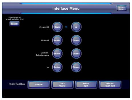
Two buttons adjacent to the *Cresnet ID* and its displayed hexadecimal number, **Down** and **Up**, decrease and increase the Cresnet ID by one, respectively.
