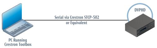
The **RS-232** port on the DVPHD connects to the serial port on the PC via a serial cable (Crestron STCP-502 or equivalent):
