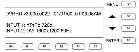
The device, firmware version, date and time are listed across the top of the screen. Each input and the type of video detected is listed beneath. To scroll through the list of inputs press **B7** and/or **B8**.
