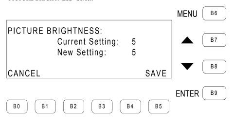
**NOTE:** The "PICTURE CONTRAST", "PICTURE SATURATION", "PICTURE HUE", "RED", "GREEN", and "BLUE", "Detail Enhancement", "Noise Reduction", "Noise Threshold", "V Size", "H Size", "X Position", "Y Position", "Phase Coarse", and "Phase Fine" screens are the same as the "PICTURE BRIGHTNESS" screen.
