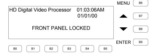
To unlock the front panel, press the **ENTER** button (**B9**). The "UNLOCK CODE" screen is displayed.
