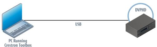
The **COMPUTER** port on the DVPHD connects to the USB port on the PC via the included Type A to Type B USB cable:
