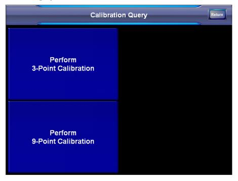
Touch **Touch Screen Calibration** on the "Main Menu" and then either **Perform 3-Point Calibration** or **Perform 9-Point Calibration** on the Calibration Query menu. Cross hairs appear in various places depending on which calibration method chosen. Touch the center of each cross hair as they appear until calibration is complete and the display returns to the "Main Menu".
