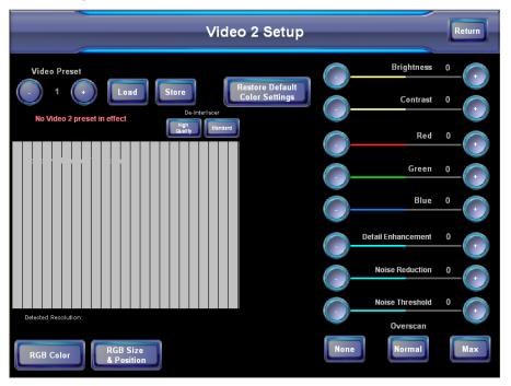
When **RGB Size & Position** is selected, the auto calibration, size and position and phase controls replace the color controls at the right.
