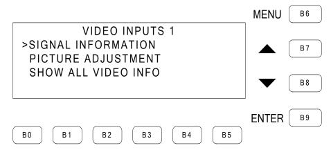
This menu provides access to the "SIGNAL INFORMATION" screen, the "PICTURE ADJUSTMENT" menu and the "SHOW ALL VIDEO INFO" menu. Press **B7** or **B8** to scroll through the selections. Press **B9** (ENTER) to open the selection.
