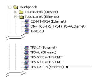
• The system tree of the control system displays the device in the appropriate slot with a default Net ID or IP ID as shown in the following illustration.
