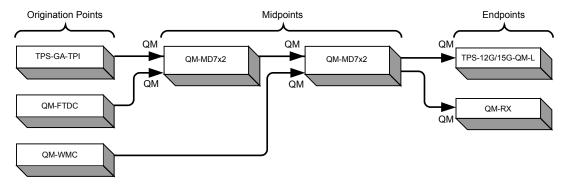
The TPS-GA-TPI is an origination point. Therefore, in a QM system, it would be positioned as shown above.
