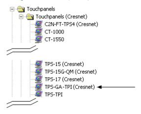
• To incorporate the TPS-GA-TPI (Ethernet) into the system, drag the TPS-GA-TPI from the Touchpanels | Touchpanels (Ethernet) folder of the *Device Library* and drop it in the *System Views*.
