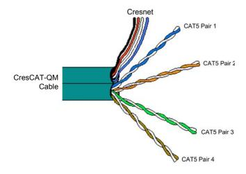
**NOTE:** Do not untwist the two wires in a single pair for more than 1/3-1/2" (0.84-1.27 cm) when making a connection. The twists are critical to canceling out interference between the wires.
