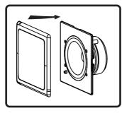
**5.** Align tabs on snap-fit grille with slots in baffle, gently press grille into place.
