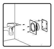
3. Install the RF31-EZ into the installer supplied junction box using included fasteners.
