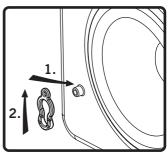
4. Attach grille safety clip by placing the large end of the clip over snap-fit post (1), then sliding clip until small end snaps into place around post (2).
