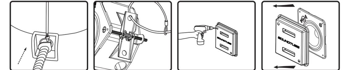
5. Feed speaker wires through conduit clamp and connect with wire nuts. Push wire nuts into backcan and affix conduit clamp.
