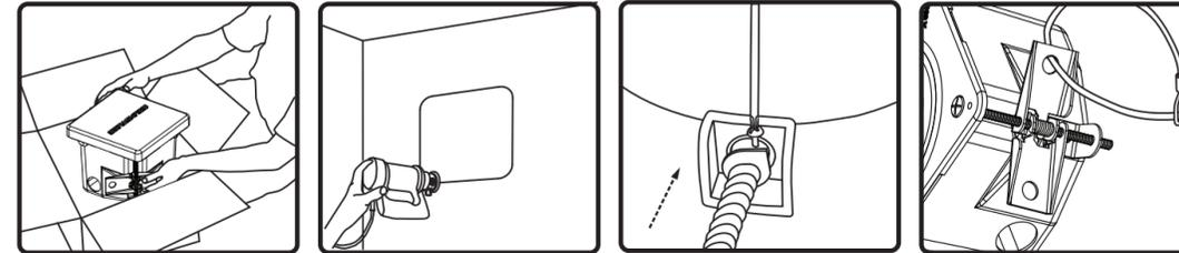
1. Unpack speaker. Leave paint mask in place until after speaker is installed or painting is complete.
