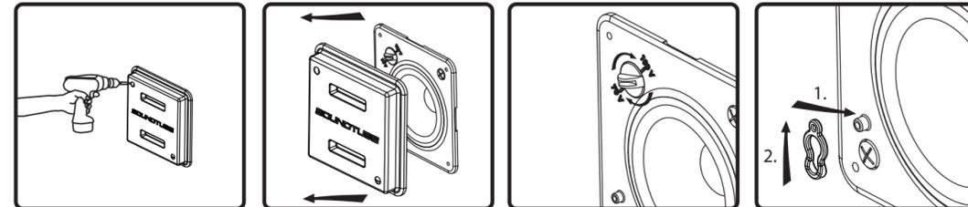
5. Insert speaker in hole. Tighten the two clamping screws. **DO NOT OVERTIGHTEN**.
