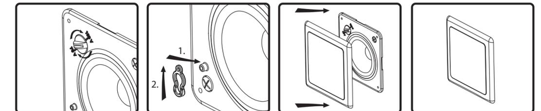
9. Adjust tap switch to proper setting. Switch is preset to the highest setting in the 70.7-volt mode.
