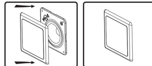
9. Align tabs on snap-fit grille with slots in baffle, gently press grille into place.
