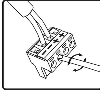
**6.** Connect signal wire to four-pin Euroblock plug. Use inside positive and negative inputs for either voice coil or distributed systems. For daisy chaining, use outside positive and negative terminals. Tighten unused terminal screws.
