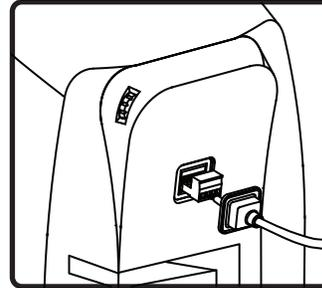
**7.** Insert four-pin Euroblock jack on rear of speaker. Connectors are keyed for polarity.
