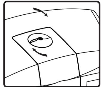
**11.** Position speaker at the desired angle and secure with the clamp knob. As a security feature, an included 5 mm Allen hex key is required for loosening the clamp knob and readjusting the speaker position angle.
