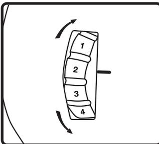
**9.** Select the desired setting on the rear-mounted tap switch. Use table on page 1 to choose appropriate tap number based on system voltage, and desired power draw.
