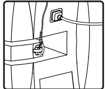
**8.** Clip snap link safety cable to eyebolt on back of cabinet.
