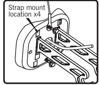
**4.** Thread safety cable (included) through mounting screw and securely fasten mounting plate to surface (user must supply fasteners). Mounting bracket may also be strap-mounted to pole or appropriate anchor point. **The max. strap width is 0.5 in / 12.7 mm.**
