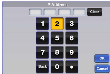
Figure 9. Numeric Pad for Setting IP Addresses
