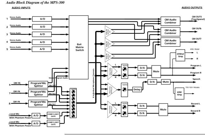
**NOTE:** The MPS-300-70V and MPS-300-100V amplify the **SPEECH** output audio path while the MPS-300 amplifies the **PROGRAM** output audio path.
