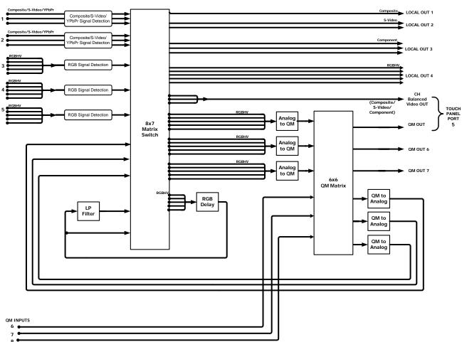
LOCAL OUT 1 and LOCAL OUT 2 can be combined to one component output. LOCAL OUT 3 can be used for composite, S-video, or component video. The MPS-300 does not convert input signal formats.
