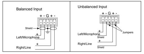
Typical Balanced/Unbalanced Outputs
