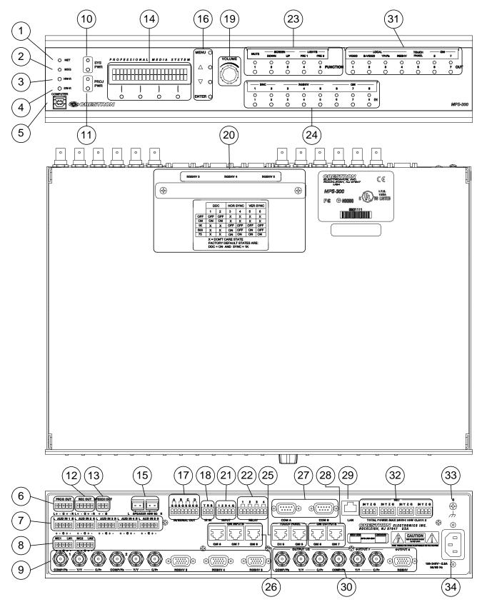
**MPS-300 Buttons and Ports**
