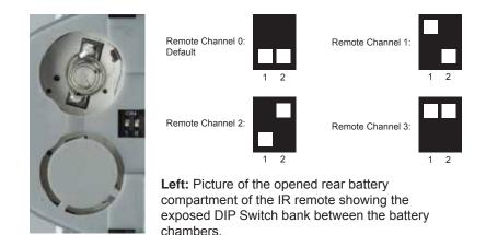
It is important that the IR channel on the Remote Control unit, matches the IR channel set on the GefenPRO 16x16 DVI Matrix. For example, if both DIP switches on the IR Remote Control unit are set to IR channel 0 (both DIP switches down), then the GefenPRO 16x16 DVI Matrix must also be set to IR channel 0. See page 25 on how to change the IR channel on the GefenPRO 16x16 DVI Matrix.
