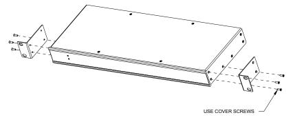
4. Repeat procedure (steps 1 through 3) to attach the remaining ear to the opposite side.
