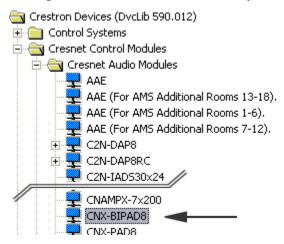
• The system tree of the control system displays the device in the appropriate slot with a default Net ID as shown in the following illustration.
