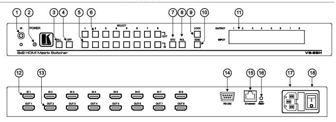
Figure 1: VS-88H 8x8 HDMI Matrix Switcher
