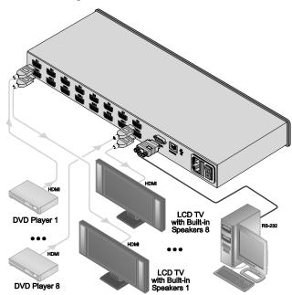
Figure 2: Connecting a VS-88H 8x8 HDMI Matrix Switcher
