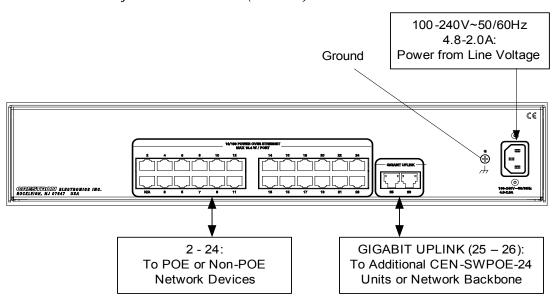
**NOTE:** Ensure the unit is properly grounded by connecting the chassis ground lug to an earth ground (building steel).
