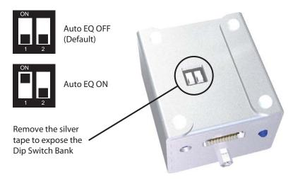
By default, both Dip Switches should be in the off position as shown above. To enable the Auto EQ, please flip Dip Switch 1 to the ON position. You must then proceed to manually adjust the EQ by turning the EQ trim pot on the front of the unit in small increments. It is important to turn the dial in very small increments as the "sweet spot" at which all video noise is eliminated can be very small.
