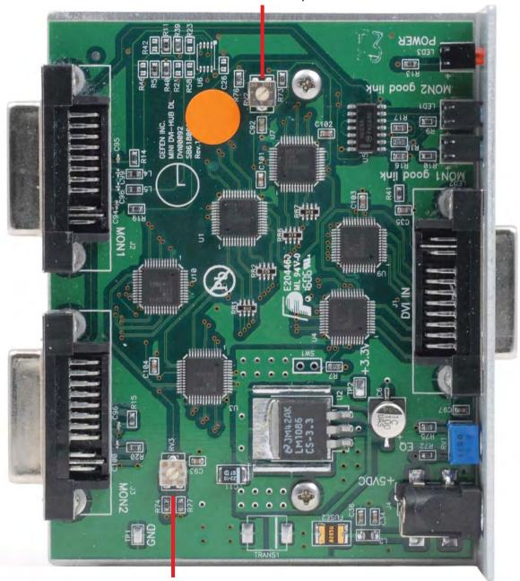
Internal Equalization Knob for DVI Output 2
