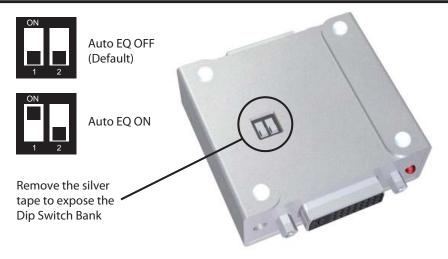
By default, both Dip Switches should be in the off position as shown above. To enable the Auto EQ, please flip Dip Switch 1 to the ON position. You must then proceed to manually adjust the EQ by turning the EQ trim pot on the front of the unit in small increments. It is important to turn the dial in very small increments as the "sweet spot" at which all video noise is eliminated can be very small.
