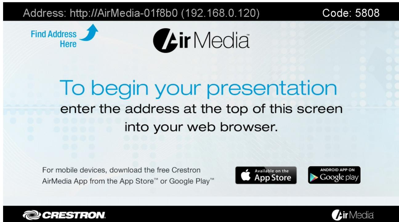
1. On the computer, open a Web browser and navigate to the Web address or the IP address that is displayed on top-left of the AM-100 welcome screen. The download screen is displayed.
