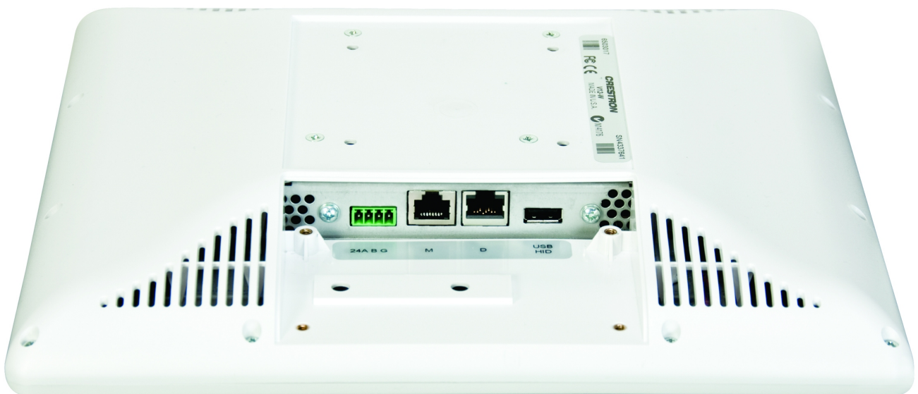
V-Panel Physical View (Rear Showing Connector Ports)
